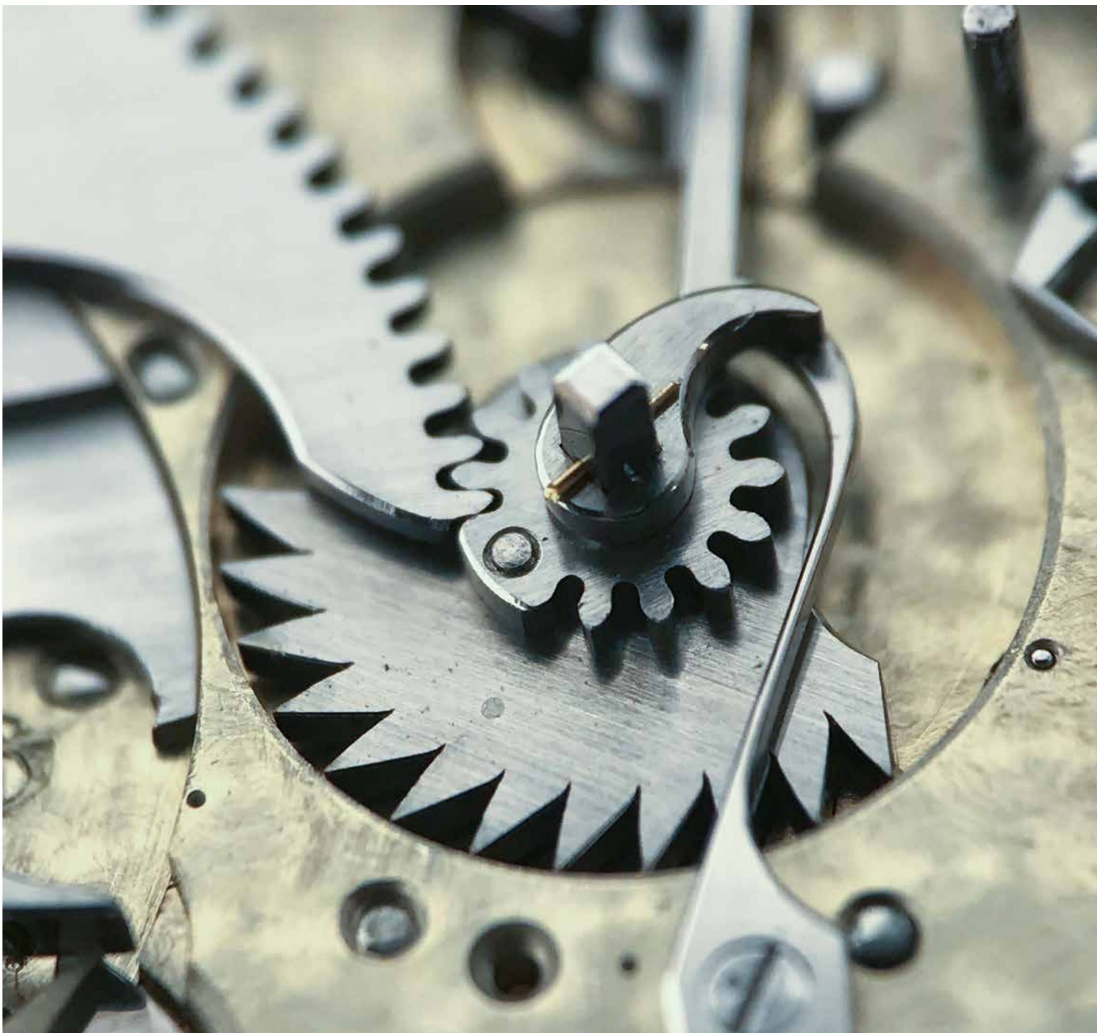
The small snail on top of the hour rack drives the 5 minute rack shown below.
